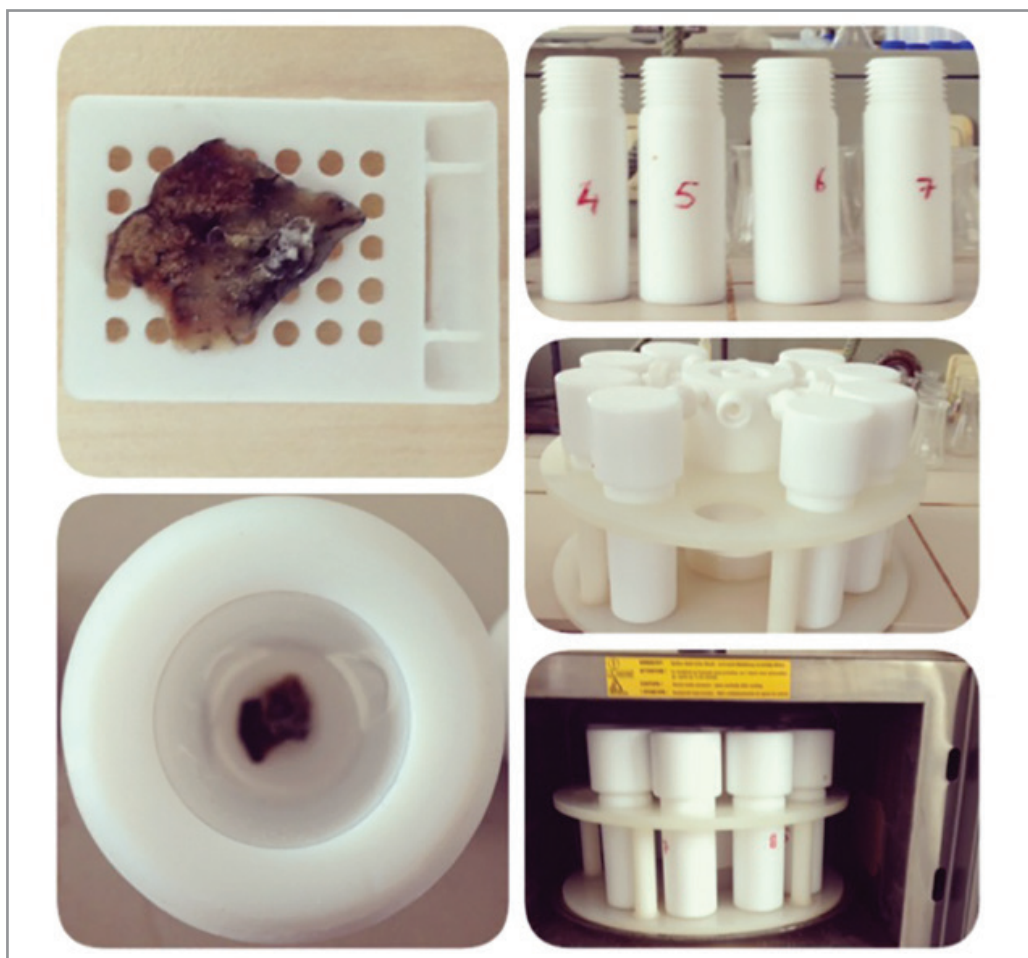
Figure 1. Acid is added to the tissue samples and placed in microwave oven.
